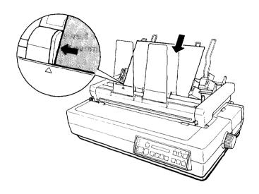
3. Press **the LOAD/EJECT** button to load the sheet. (If your document is more than one page long, the next sheet is automatically loaded from the cut sheet feeder's paper supply.)
